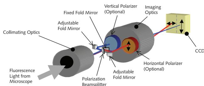
Figure 2. Operation of the DV2 fluorescence polarization imaging system.
