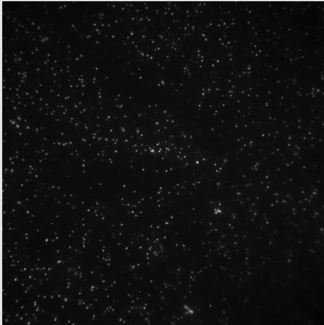
Alumina ( $\text{Al}_2\text{O}_3$ ) coated gallium phosphide (GaP) nanowires functionalized with biotinylated BSA (bovine serum albumin). Streptavidin labelled with three fluorescent dyes (FITC, TRITC and Cy5), imaged under 100x magnification.
