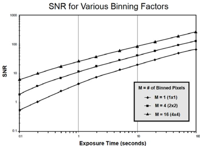
Figure 4. Binning can improve the SNR of a device, allowing the imaging system to reach a photon-noise-limited signal more quickly.
