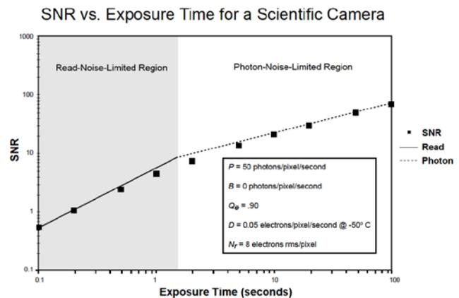
Figure 2. Under low-light-level conditions, high-performance CCD camera systems become photon-noise limited at shorter exposure times.
