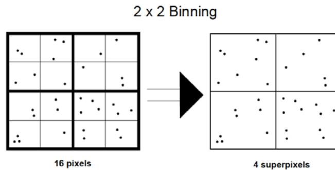
**Figure 3.** The charge from adjacent pixels in a CCD can be combined during readout to improve the signal-to-noise ratio. Note that the higher SNR comes at the expense of spatial resolution.
