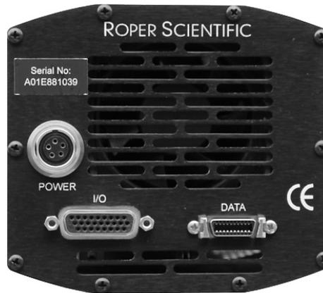
The following connectors are located on the back of the camera.
