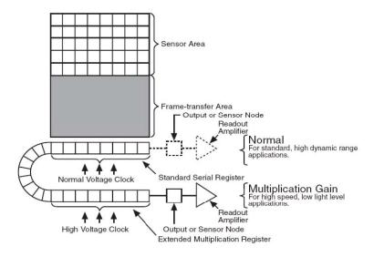
Figure 1. Cascade II CCD
