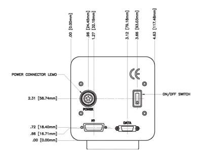
Figure 22. Cascade II Back camera view
