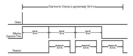
Figure 10. Timing diagram for Overlap Mode when exposure time > readout time
