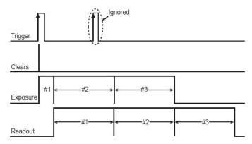
Figure 17. Trigger-first Mode timing diagram: Overlap mode
