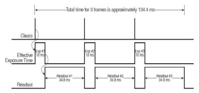
Figure 13. Timed Mode timing diagram: Non-overlap mode
