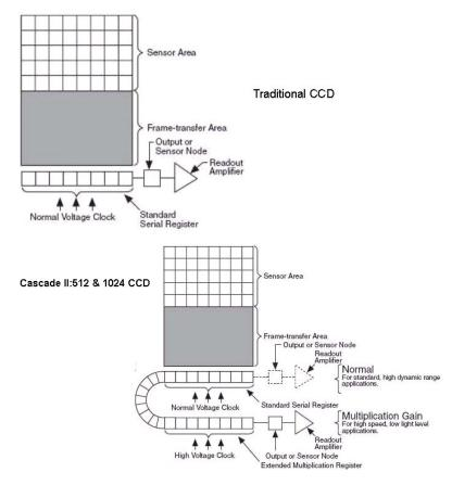
Figure 5. Comparison of traditional CCD and Cascade CCD array structures
