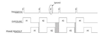
Figure 15. Strobe Mode timing diagram: Non-overlap mode
