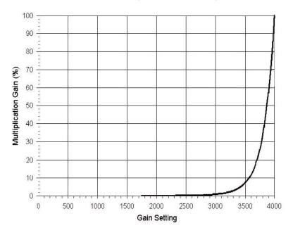
Figure 6. Gain setting vs. Charge multiplication gain
