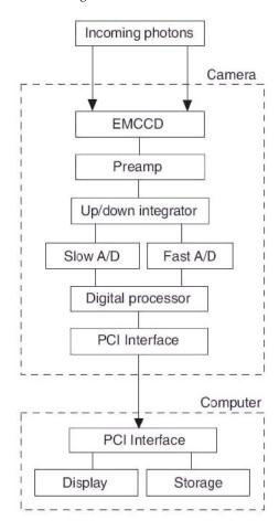
Figure 4. Block diagram of Cascade II system
