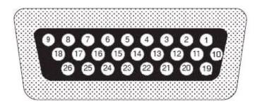
Figure 26. I/O connector pinouts
