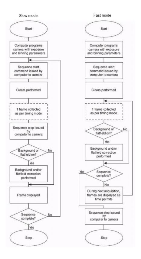
Figure 19. Flow charts of Slow and Fast mode operation
