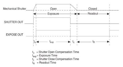
Figure 12. External Shutter timing diagram
