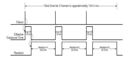
Figure 11. Timing diagram for Non-Overlap Mode
