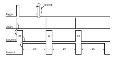
Figure 18. Trigger-first Mode timing diagram: Non-overlap mode
