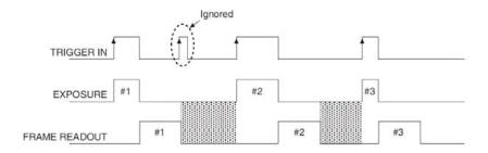
Figure 16. Bulb Mode timing diagram: Non-overlap mode
