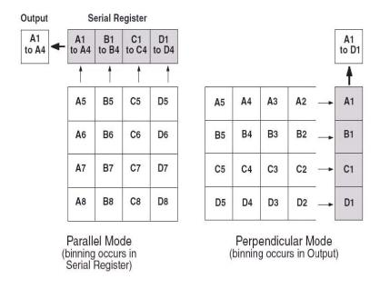
Figure 8. Binning and array orientation
