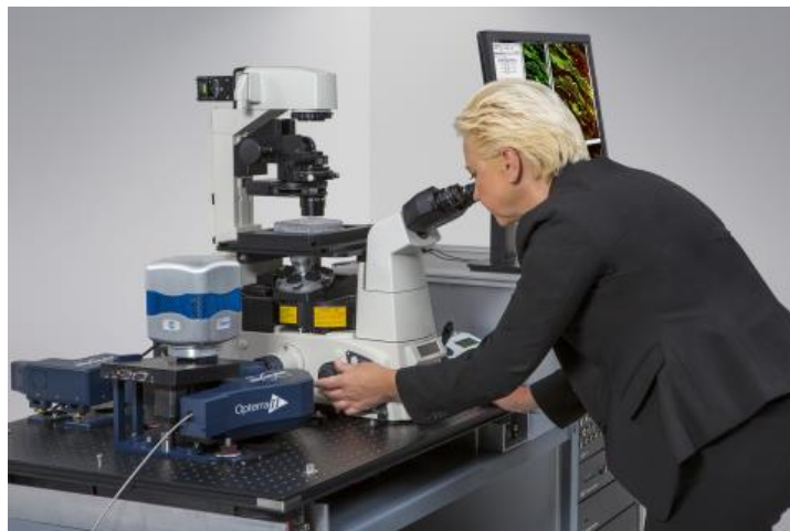
Figure 3: Bruker Opterra II on a Nikon TiE equipped with a Photometrics Evolve 512 Delta (From Bruker)
