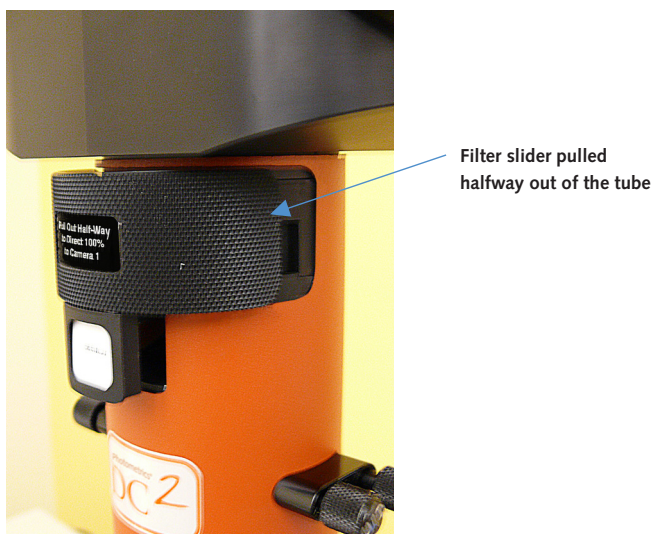
Figure 2. Filter cube in Bypass Mode position.
