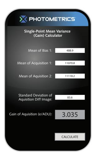
When light is detected by the camera, it needs to be processed and quantified, so that the data displayed to the user is accurate and precise. This quantization process is the application of the camera system gain. This system gain can vary from camera to camera, depending on a few factors ranging from camera electronics to CCD properties. To be accurate in the quantization process, each camera needs to be benchmarked for its specific system gain.
