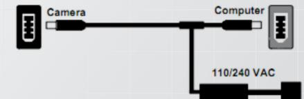
**WARNING:** Your camera will be damaged if the IEEE 1394 cable is not plugged into **BOTH** the computer **AND** the camera correctly. The cable connectors only fit one way and should slide easily into ports as shown below. Plugging the cable in improperly will void your warranty and require the camera to be returned to QImaging for repair.
