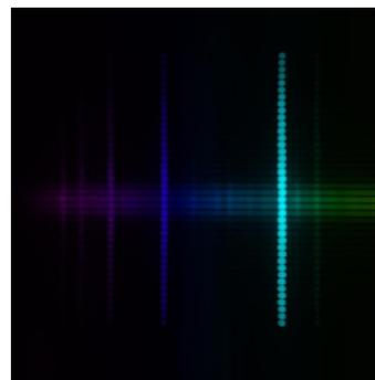
**Figure 2:** The left figure shows a spectrum at middle fiber low resolution setting. The right figure shows light from the plasma beam imaged on a fiber array and the spectra imaged with the Prime 95B. Each fiber corresponds to a certain plasma position of the beam, i.e. a radial profile of the beam is measured. The highest peak corresponds to a Balmer beta line (488 nm,  $n=4 > n=2$ ).
