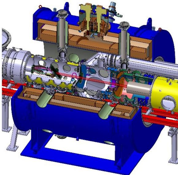
**Figure 1:** A side cutaway view of the linear plasma generator Magnum-PSI. The plasma (magenta-colored beam) exhausted by the plasma source (right side) is confined by the max 2.5 Tesla magnetic field (super conductive magnet (dark blue)) and deposited on a sample (power flux <math><40 \text{ MW/m}^2</math> continuously and transients >1GW/m<sup>2</sup>). Different diagnostics are used for measuring the plasma conditions.
