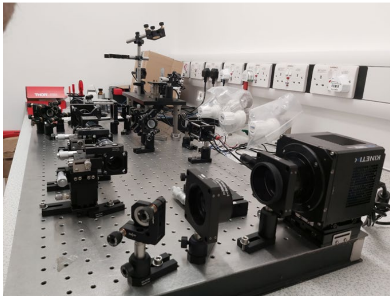
Figure 1: Image of the Kinetix sCMOS set up on the OPM light sheet imaging system, optimised for high speed single molecule imaging of live cells.
