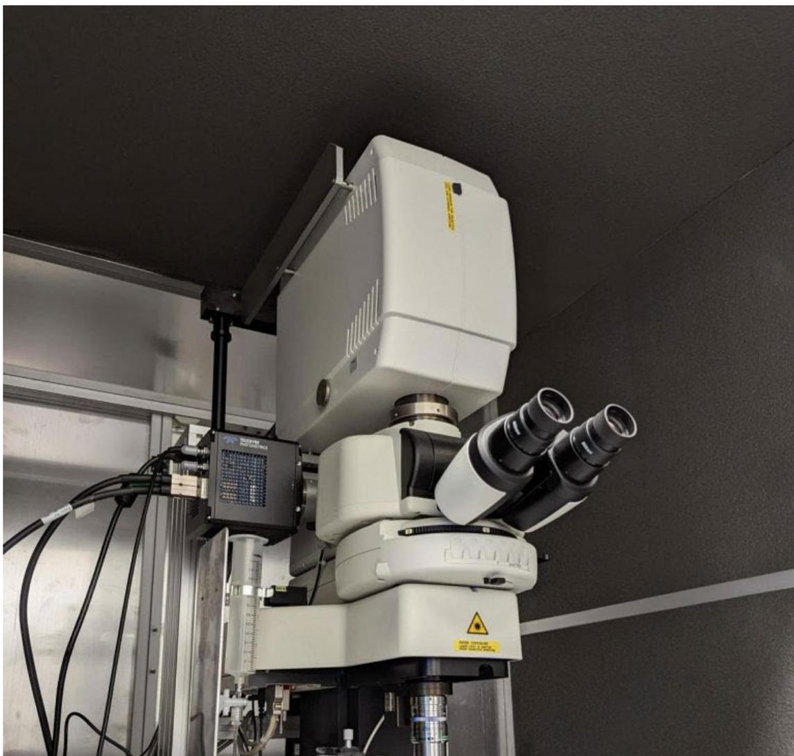
**Figure 1:** The Kinetix sCMOS connected to an imaging system within an electrophysiology cage, set up for electrophysiology and/or voltage imaging experiments.
