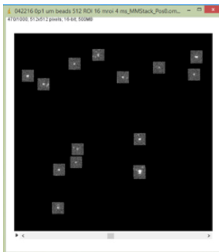
Figure 5b. Example of a 512x512 region, with PrimeLocate configured to find the 16 brightest regions, and return them as 31x31 pixels patches
